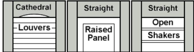
**Louver Shutter Profile:** Select the desired combination of louvers, raised panel(s), and shaker components in one color or a combination of two colors. (Double width not reflected in drawing.)
